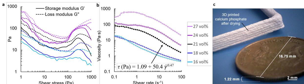
Fig. 1 – (a-b) Rheological curves of inks comprising 16 to 27 vol% CaP. In (b), the equation corresponds to the Herschel-Bulkley model for the ink with 21 vol% CaP. (c) Optical image of CaP printed from 21 vol% CaP ink, placed next to a Singapore 5-cent coin.
