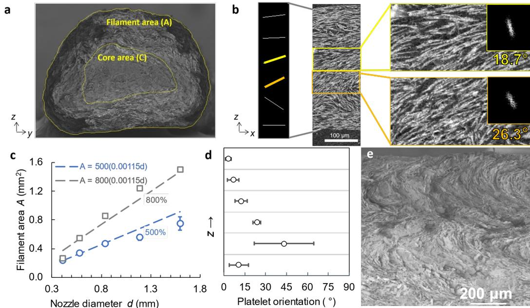
Fig. 2 (a) Filament cross-section showing concave fracture surface. (b) Gradient platelet orientation in filament. (c) Filament cross-section area at flow rate multiplier 500% and 800%. (d) Typical platelet orientation in a filament. (e) Gradient microstructure in multi-layer structure.
